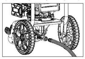
The minimum recommended length for the water supply pipe is 10 meters (but not more than 25 meters) with a diameter of 12.5 mm to avoid back pressure and any potential damage to your appliance. Make sure it can withstand water and a maximum pressure of 10bar (0.1Mpa). If you want to connect your device to other water sources, make sure the maximum water inlet pressure is 10bar (0.1Mpa).
