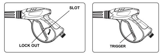
WARNING Kickback forces result from pressing the trigger! Therefore, always hold the spray gun with
